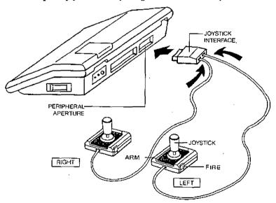
ARM and FIRE button. The joystick interface allows your VZ300 to support the joysticks.
