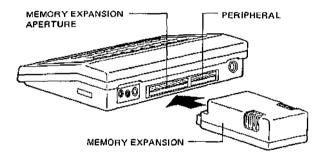
To check that the extra memory is correctly inserted, you type in PRINT PEEK (30897) and press the RETURN key, which should give you an answer of 255. Then, if you type in PRINT PEEK (30898) and press RETURN, you'll get 247.
