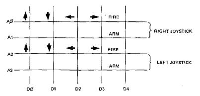
You use the IN instruction to read the joystick whose address ranges from hexadecimal 20 to 2F. All you have to do is write a program to scan the address lines, and check which data bit has become zero.
